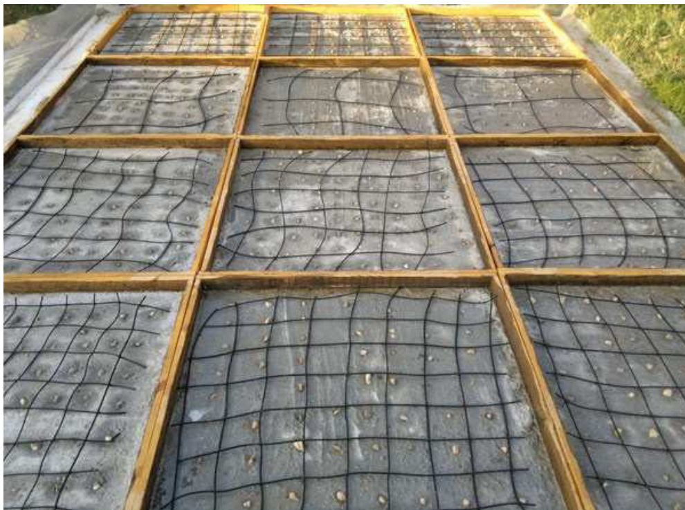
Figure 3-23: Slabs with different RLDPE contents
