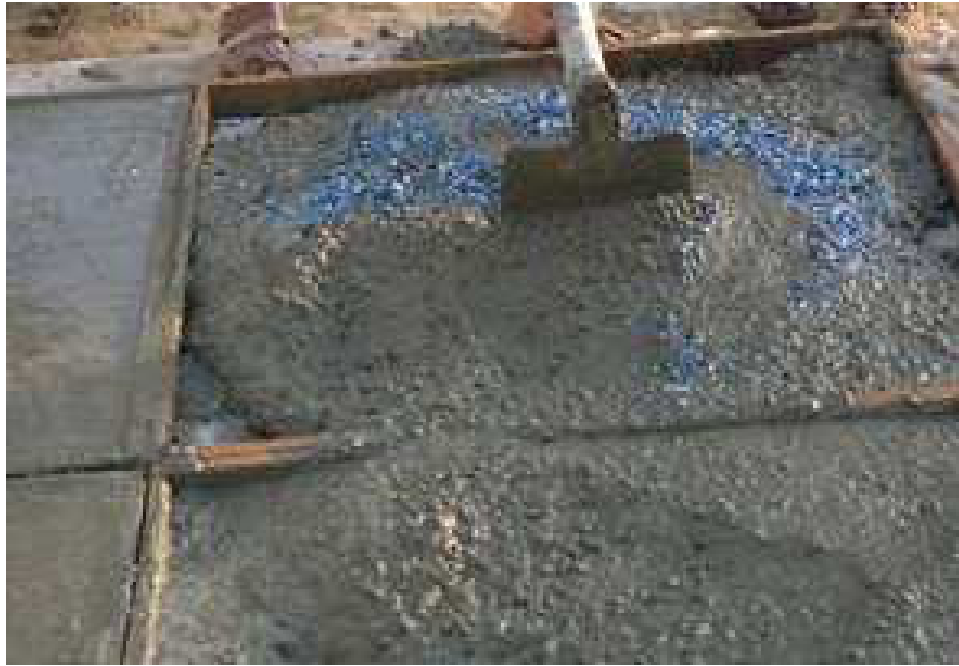
Figure 3-22: Filling the second template with concrete for different RHDPE contents.
