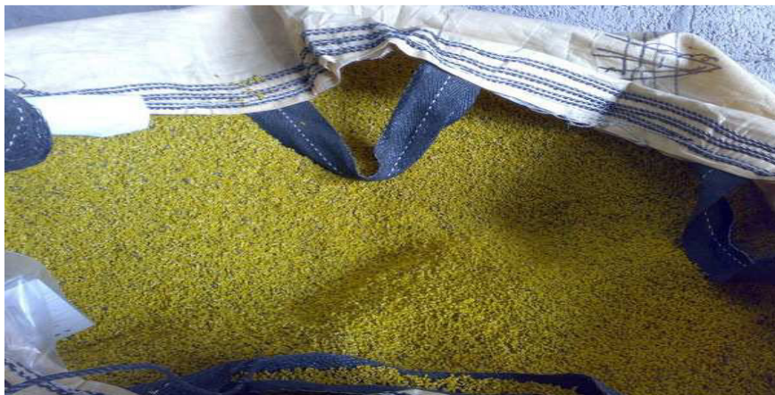
Figure B.8: Shredded Pieces for Recycled high-density polyethylene (RHDPE).
