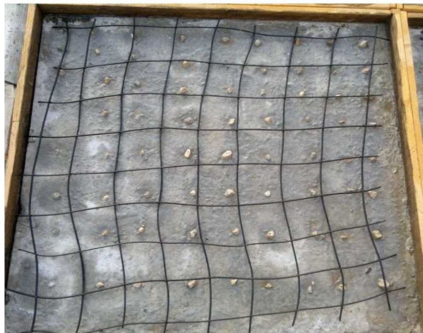
Figure 3-8: 0.3% RLDPE fibers as secondary reinforcement.
