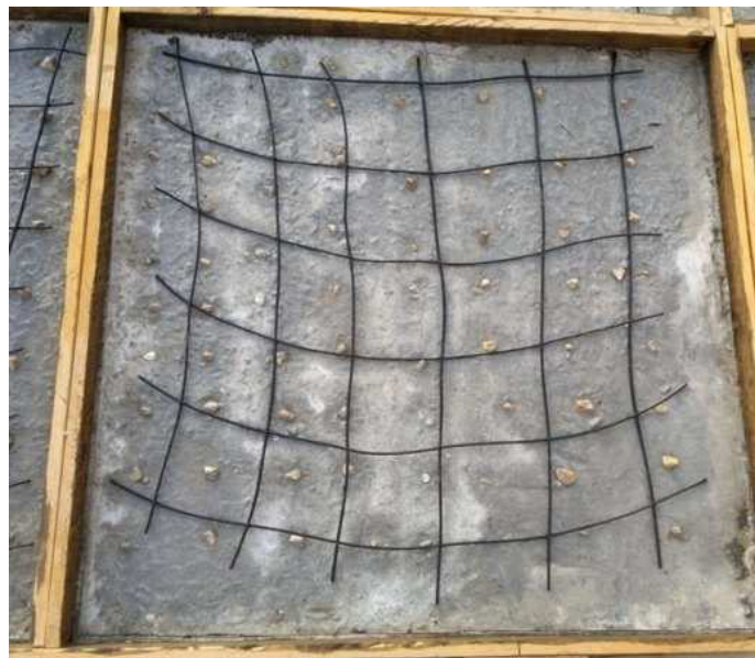
Figure 3-7: 0.2% RLDPE fibers as secondary reinforcement.
