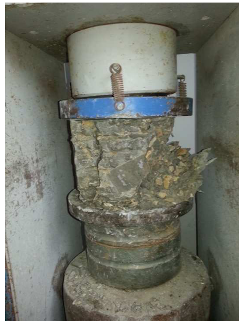
Figure 4-4: Plastic concrete cubes failure
