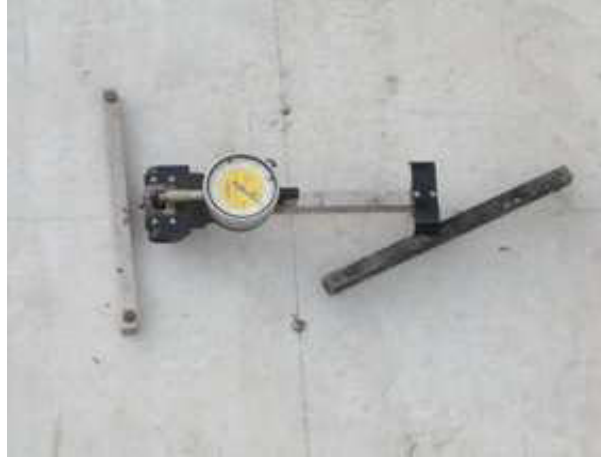
Figure 3-13: Demec gauge datum discs
