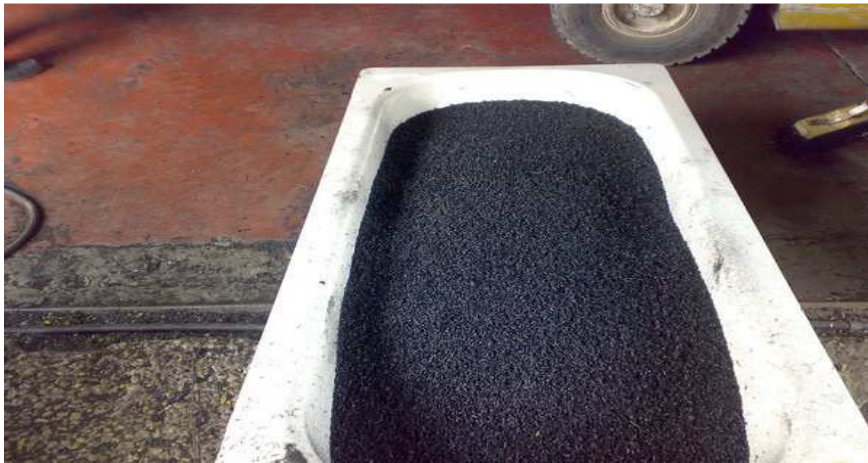
Figure B.8: Shredded Pieces for Recycled Low-density polyethylene (RLDPE).
