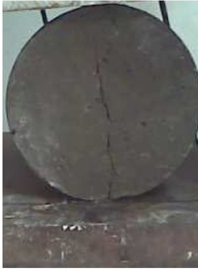
Figure 4-6: Failure pattern of control concrete
