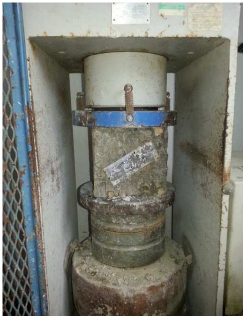
Figure 4-3: Control concrete cubes failure
